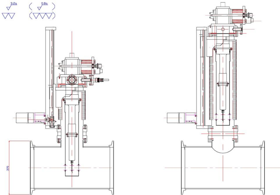
Fig. 5: Schematic of target chamber placed at beam transport line at 3-GeV synchrotron. Left and right-hand side show irradiation and evacuation position of the sample, respectively. The similar structural chamber will be employed with placing at the beam transport line to the MR abort beam dump.
