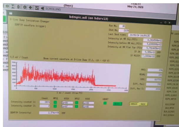
Fig. 2. The first shot to B-line measured with Ion Chamber (IC) at a beam-dump. Horizontal is time in millisecond while vertical is IC counts.
