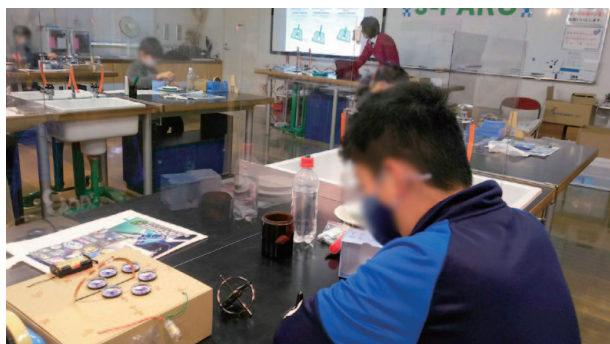
Participant observing magnetic field created by electric current (magnetic lines of force)
