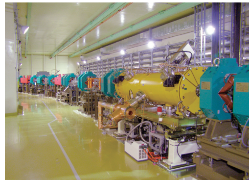
BL to RCS. One SDL unit is used as debuncher until ACS is installed.
