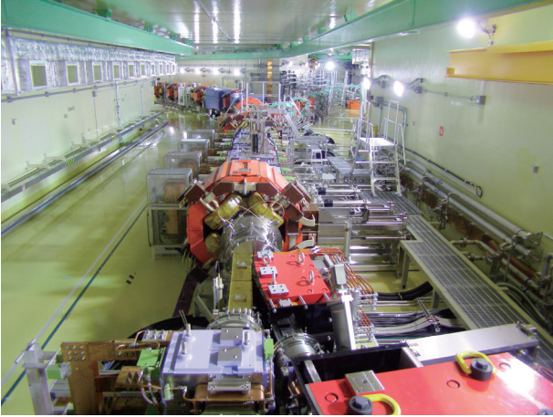
Injection region. The beam comes from the upper-right corner. The charge exchange foil system is located in the middle. The BL to H0-dump is below to the right.
