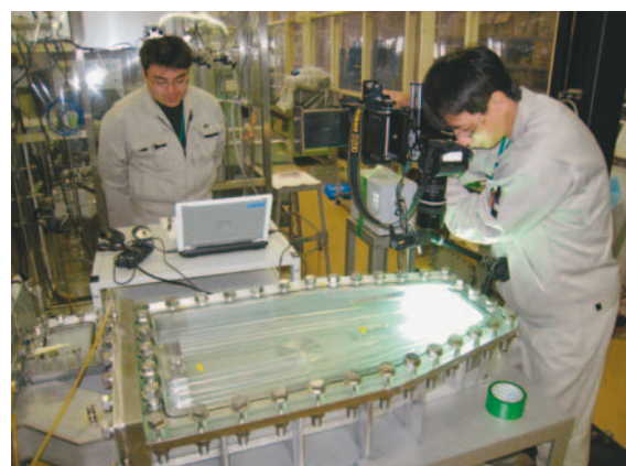
Photo 2. Target model used for performance tests of microbubble injection device.
