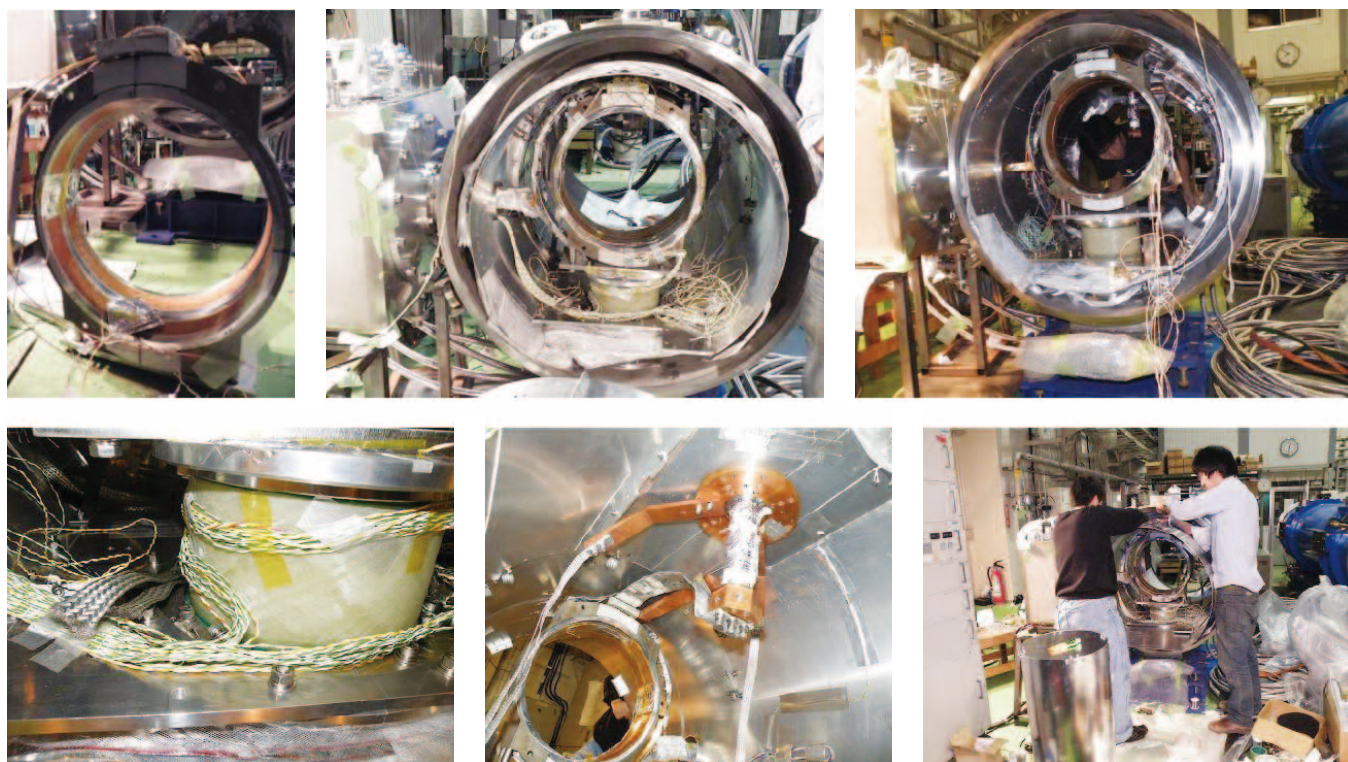
Photo 1. Cryogenics setup for testing super omega curved solenoid model coil.
