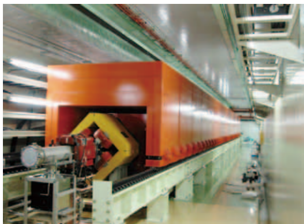
Photo 2. The 3-50 BT collimator section with the newly installed gate-shaped iron shields.
