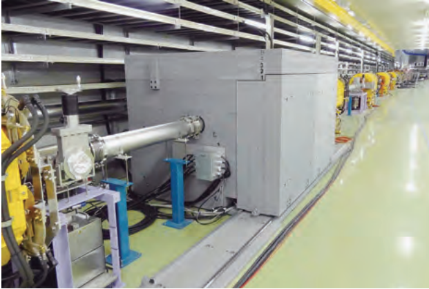
Fig. 4.6. New collimator system installed in the SX straight section.
