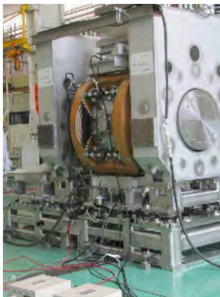
Fig. 15. The vacuum chamber of the positron separator and the cryostats of the superconducting coils of the axial focusing solenoid.
