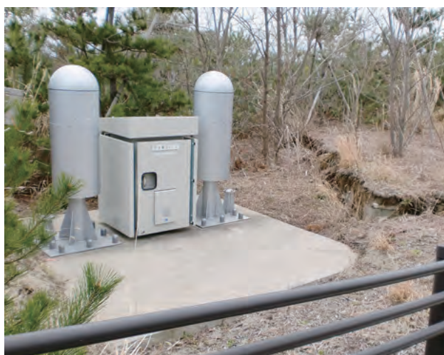
Photo 3. Radiation area monitor above the 3NBT Dump.
