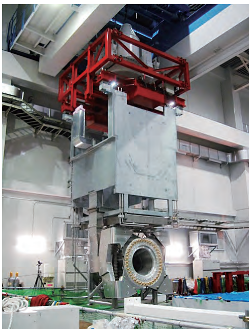
Fig. 3. The 3rd horn under transportation from the beam line to the maintenance area for inspection. All the works were done remotely due to the high residual radio-activity.
