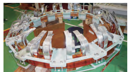
Fig. 4. The R&D coil of the capture solenoid for COMET.
