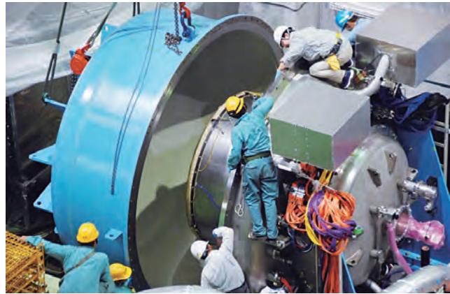
Fig. 2. KOTO personnel working on placing a cap on the calorimeter for a vacuum test.
