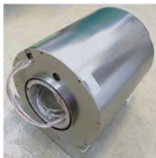
Fig. 17. A developed magnetostatic cavity. The outer dimensions of the cavity were 272 mm in diameter and 364 mm in length.
