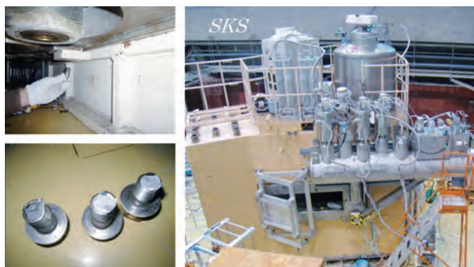
Fig. 1. The Superconducting Kaon Spectrometer (SKS) magnet with broken bolts (left).
