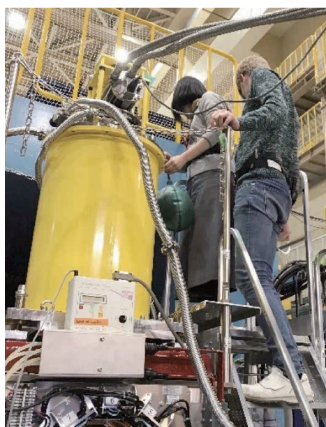
Fig. 7. Users from Toyota Central Res. Dev. Lab (Japan) and KTH Royal Institute of Technology (Sweden) are preparing the sample mounted in a cryo-furnace.
