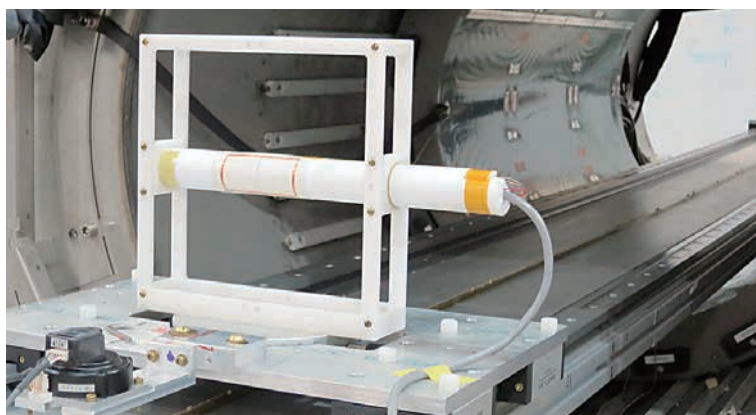
Fig. 5. Material effect measurement of a new standard probe at the ANL.
