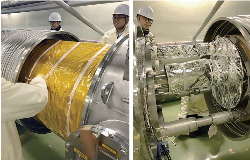
Fig. 3. Picture of the cryostat for the beam monitor before the repair works.
