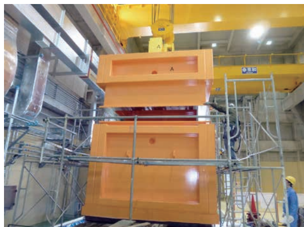
Fig. 2. Photo of the shipping container for used target vessels.
