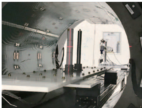
Fig. 6. Cross calibration test between KEK and US probes in the MRI magnet at the ANL.
