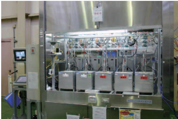
Fig. 4. Oxygen sensor calibration system under stagnant LBE condition
