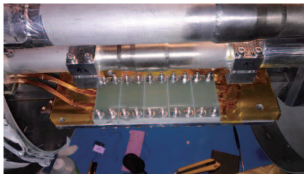
Fig. 5. Soldered splices at the interface to the protection diodes of the Muon Transport Solenoid.
