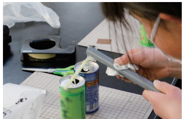
Pendulum bell generating static electricity using a PVC
