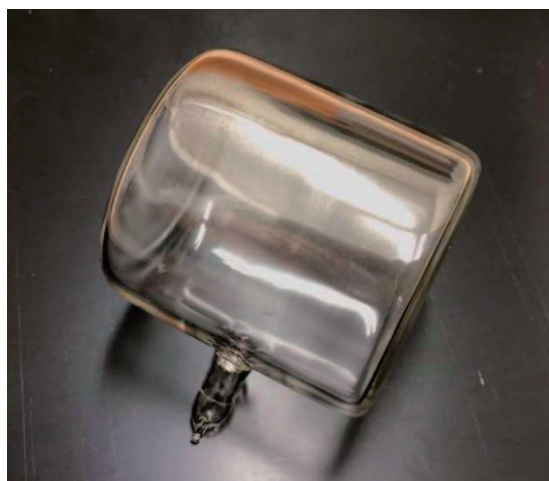
Fig. 1. The ^3\text{He} spin filter cell fabricated at J-PARC.
