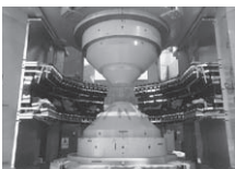
Photograph ② : The Lead Glass Calorimeter for J-PARC E16 Image credit: Sakiko ASHIKAGA
