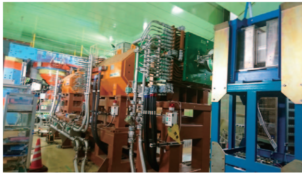
Fig. 5. The newly constructed B-line and a spectrometer (left end) for the new E16 experiment.
