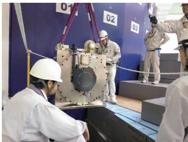
Fig. 1. Brand new T0 chopper installed into the beamline of 4SEASONS.
