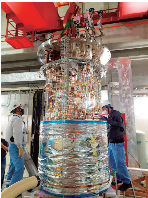
Fig. 5. Insert of the current lead box for the Pion Capture Solenoid.
