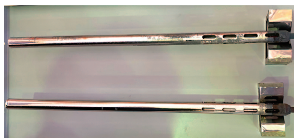
Fig. 2. Outline of specimen holders after the corrosion test operation.
