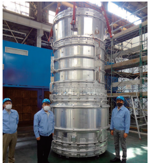
Fig. 6. The coldmass of the Pion Capture Solenoid (CSMS coils).
