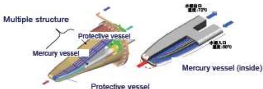
Figure 2.4: Structure of the multi-layer protective vessel for the Neutron Target. The target vessel consists of a container for mercury and a protective vessel. The protective vessel has two layers of metal walls interleaved with a helium gas layer, which is continuously monitored to detect any leakage of radioactive material and/or mercury.
