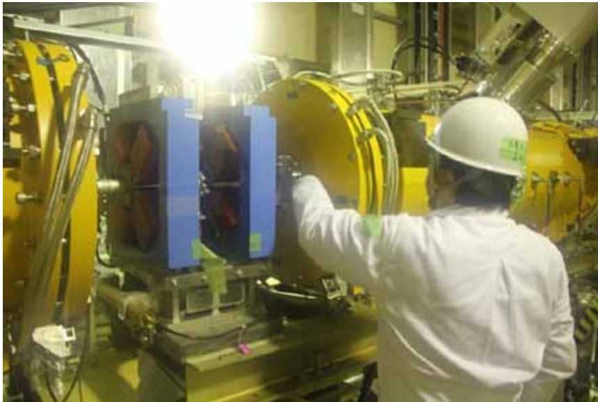
Ceramic Vacuum Current Transformers located between the cavities (upper and upper right). Over 20 of them were destroyed. Sharply bent joint bellows (right).
