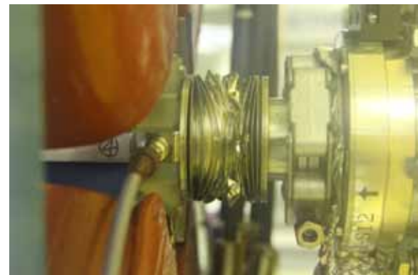
Ceramic Vacuum Current Transformers located between the cavities (upper and upper right). Over 20 of them were destroyed. Sharply bent joint bellows (right).
