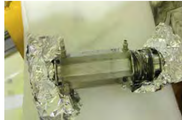
BPM (Beam Profile Monitor) extracted from Q-Magnet. Bellow was destroyed.
