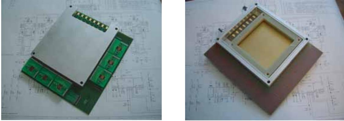
Figure 39: Bottom (left) and top (right) view of the prototype triple-GEM chambers. The location of the sensitive detector volume can be clearly seen on the right side with the location of three inner G10 carrier frames. No GEM foils have yet been glued onto those frames. The location of groups of three readout hybrids can be clearly seen on the left side.
