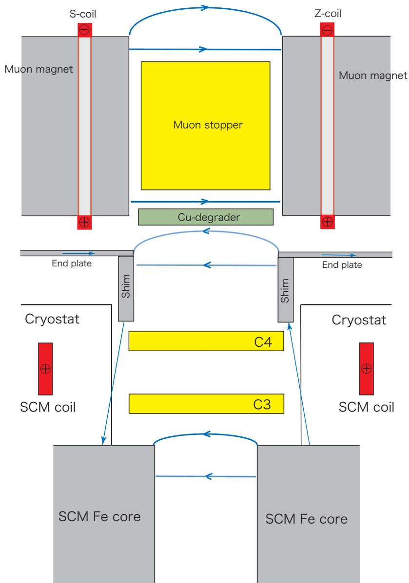
Figure 19: Schematic cross section of one sector with new muon field magnets.
