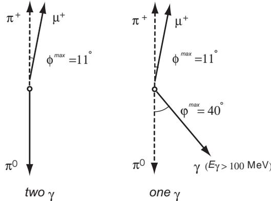
Figure 35: Angular ranges of  $K_{\pi 2-dif}$  back-to-back condition for  $2\gamma$  events compared with  $1\gamma$  events.
