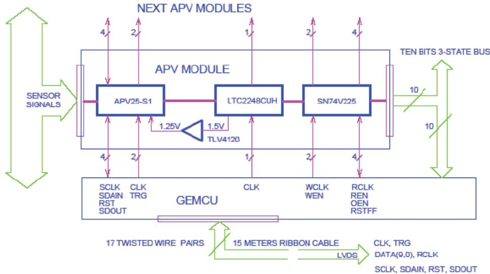
Figure 42: Sketch of the APV25 chip readout system.
