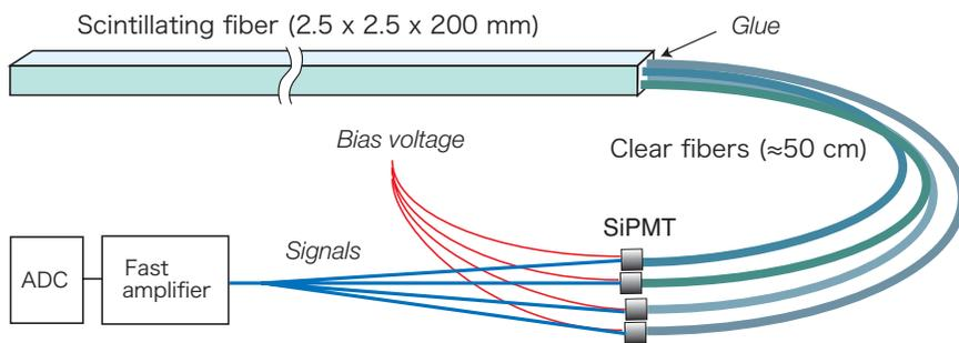
Figure 9: Schematic readout for each of the 432 fibers in the target bundle for the proposed experiment.
