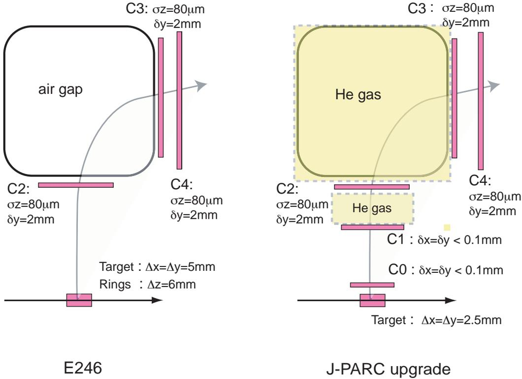
Figure 10: Schematics of the tracking system in the E246 setup (left) and the proposed setup for the J-PARC experiment (right).
