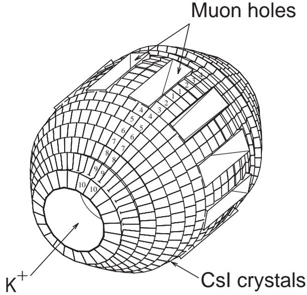
Figure 11: CsI(Tl) barrel with 768 crystal modules. There are 12 muon holes.
