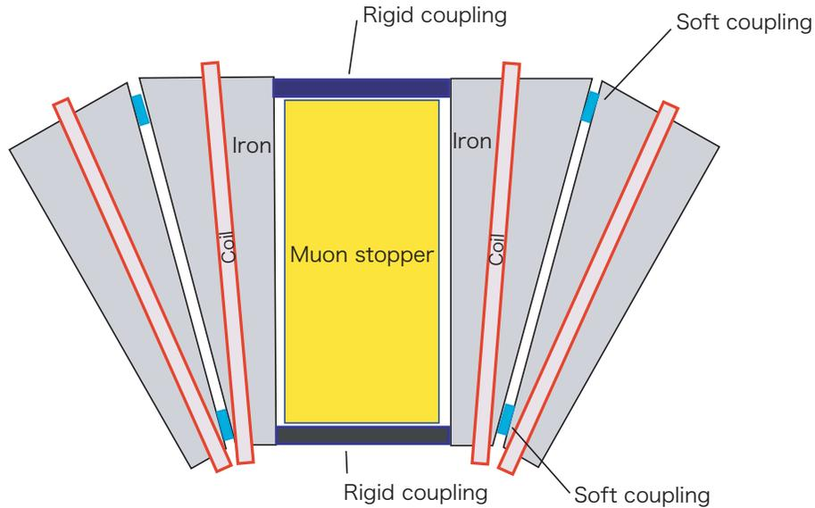
Figure 18: Schematic front view of the muon field magnet.
