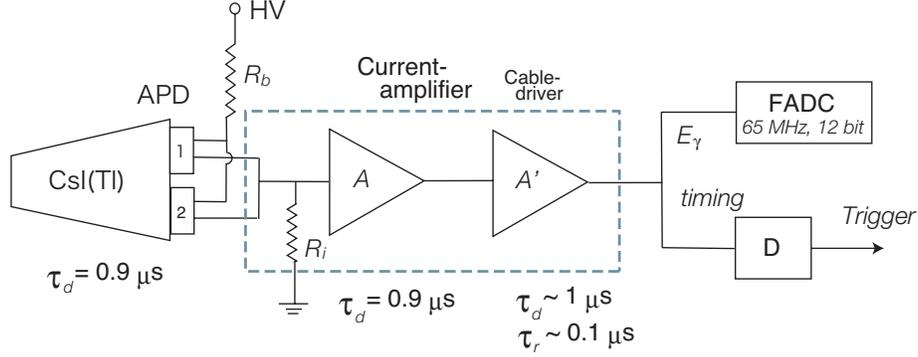
Figure 14: Readout scheme of the CsI(Tl) calorimeter using APD.
