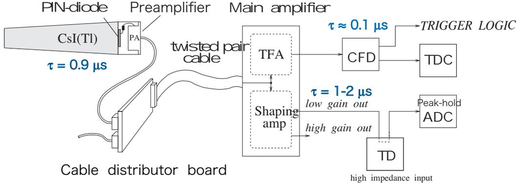
Figure 13: Current readout scheme of the CsI(Tl) calorimeter.
