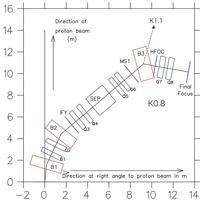
Figure 23: Layout of the 0.8 GeV/c beam.
