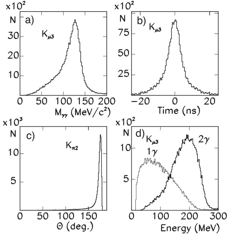
Figure 12: Performance of the CsI(Tl) detector for  $K_{\mu 3}$  and  $K_{\pi 2}$  in E246. a) Invariant mass spectrum of two photons of  $K_{\mu 3}$ , b) cluster timing distribution also of  $K_{\mu 3}$  showing the time resolution, c) opening angle distribution of  $K_{\pi 2}$  showing the angular resolution, and d) two-photon and one-photon energy spectra of  $K_{\mu 3}$  events.
