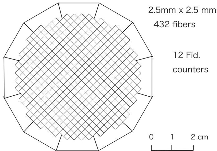
Figure 8: Scintillating fiber target for the proposed experiment. The active zone has a length of 20 cm and a diameter of 6 cm. Each of the 432 scintillating fibers has a  $2.5 \times 2.5$  mm<sup>2</sup> square cross section. The fiber bundle is surrounded by 12 fiducial counters.
