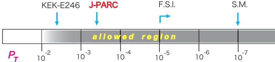
Figure 2: Experimental status of  $K_{\mu 3}$   $P_T$  physics relative to the SM prediction is illustrated. The experimental limits are in 90% confidence limits. “Allowed region” means that some of the non-SM CP violation models allow  $P_T < 10^{-2} \sim 10^{-3}$  without conflicting with other experimental limits.
