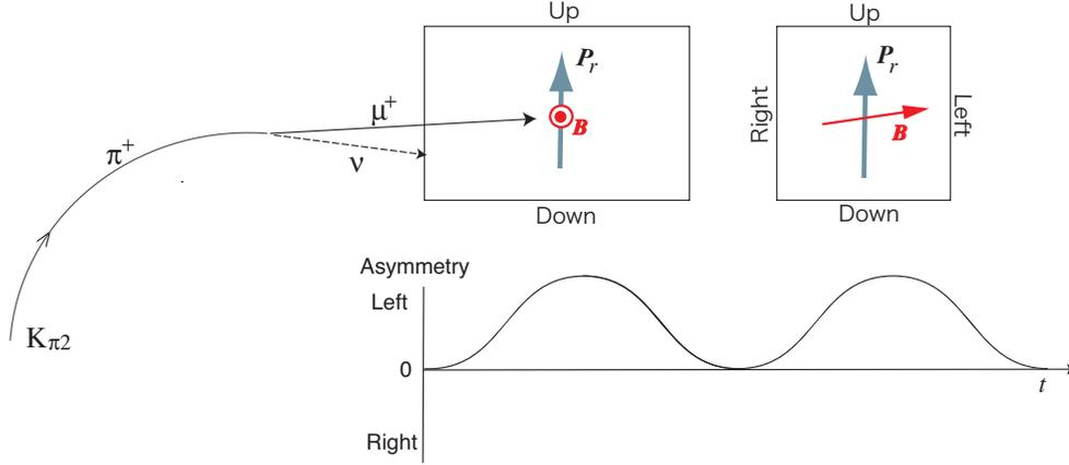
Figure 34: Calibration of magnetic field alignment using  $K_{\pi^2}^{+}$ -dif muons. Polarization with a pure radial component is generated in the stopper. The asymmetry measurement for this polarization yields Eq.30.
