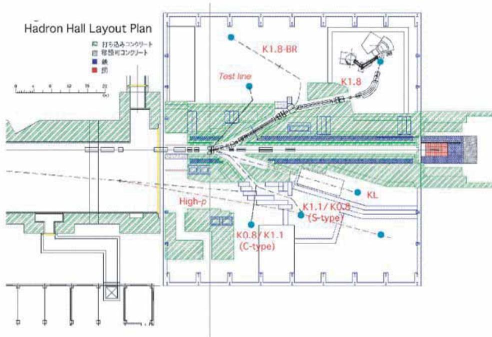
Figure 21: Layout of beamlines in the Phase-1 experimental hall
