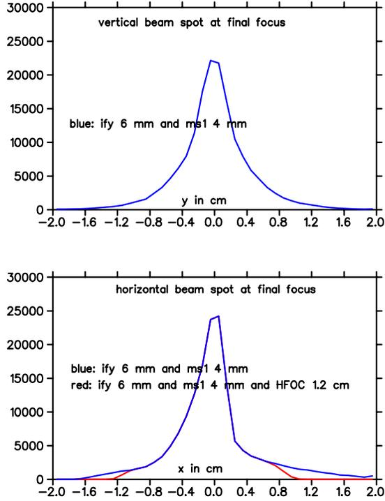
Figure 27: ZGOUBI result for the 0.8 GeV/c beam. Vertical and horizontal beam spots at the final focus.
