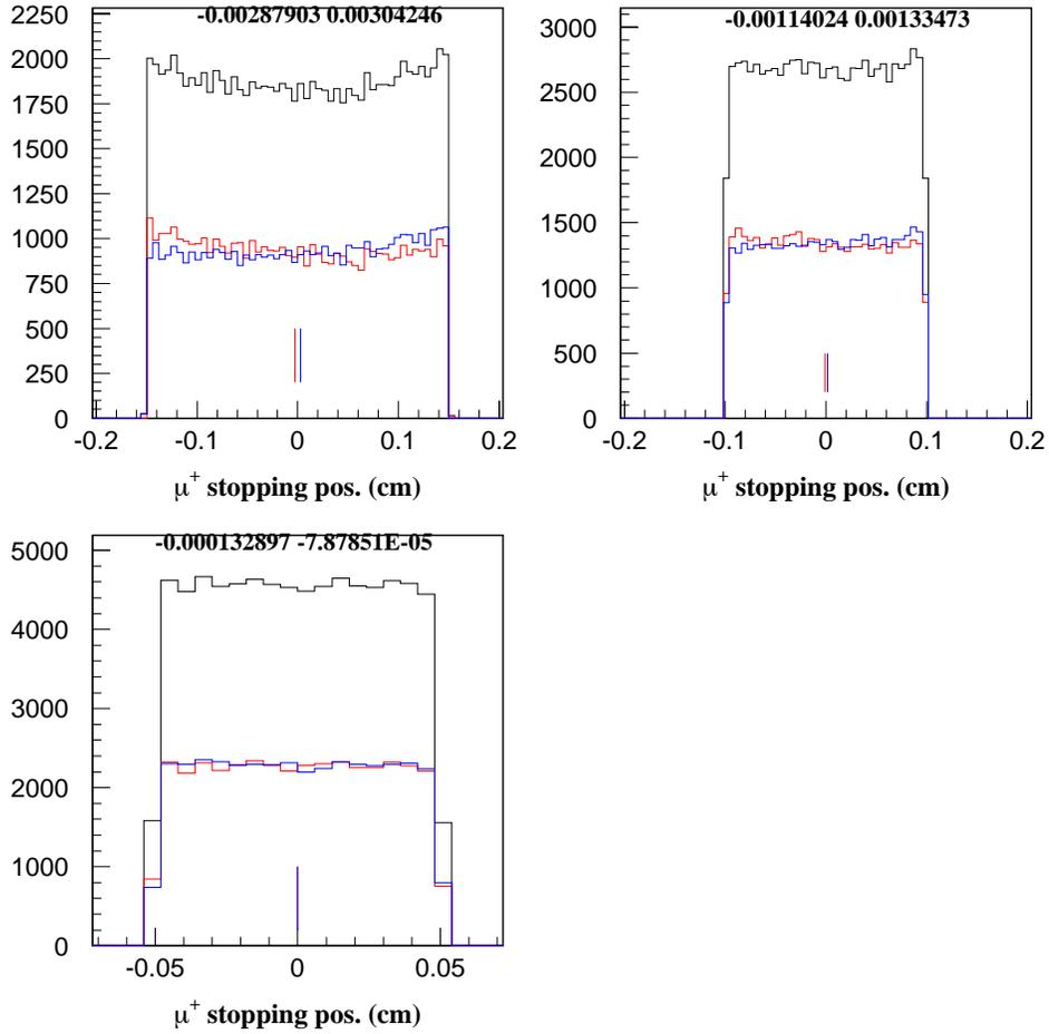
Figure 17: Muon stopping distribution across the cross-section of a plate calculated in a Monte Carlo simulation under a realistic muon incident condition. Slightly opposite gradients are seen between the two cases of left-hand side (red) and right-hand side (blue) incident muons. This difference may become a source of systematic error.
