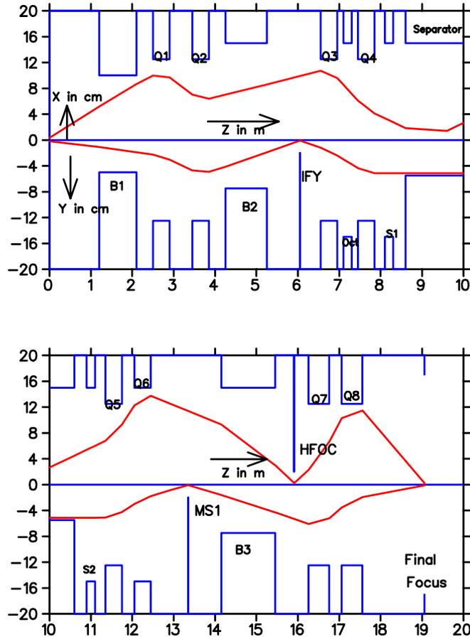
Figure 24: First order beam envelopes for the central momentum of the 0.8 GeV/c beam from TRANSPORT. The initial horizontal angle is 43 mr, the vertical angle is 9 mr. X is 3.5 mm and Y is 2 mm. All numbers indicate half widths.
