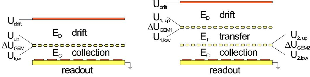
Figure 38: Schematic view of a single (left) and double (right) GEM detector.
