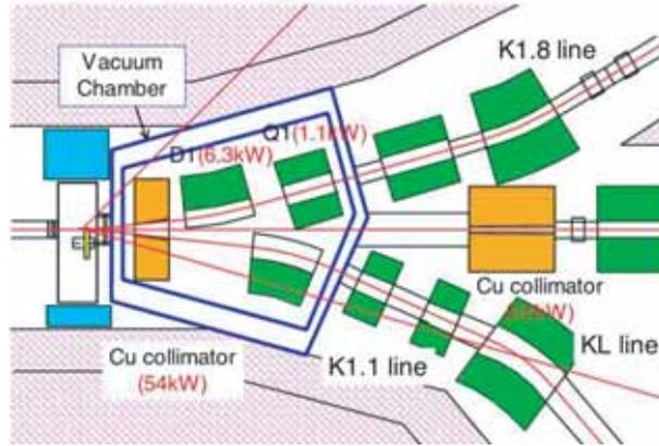
Figure 22: Almost fixed design of the target station T1 and front-end of secondary lines
