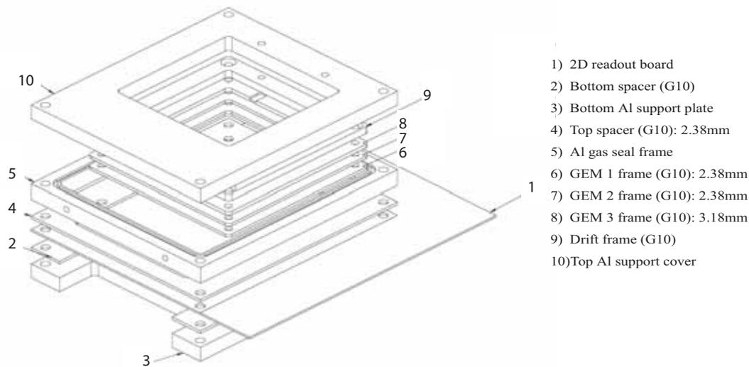
Figure 40: Exploded view of a prototype triple-GEM chamber indicating the location of various chamber elements.
