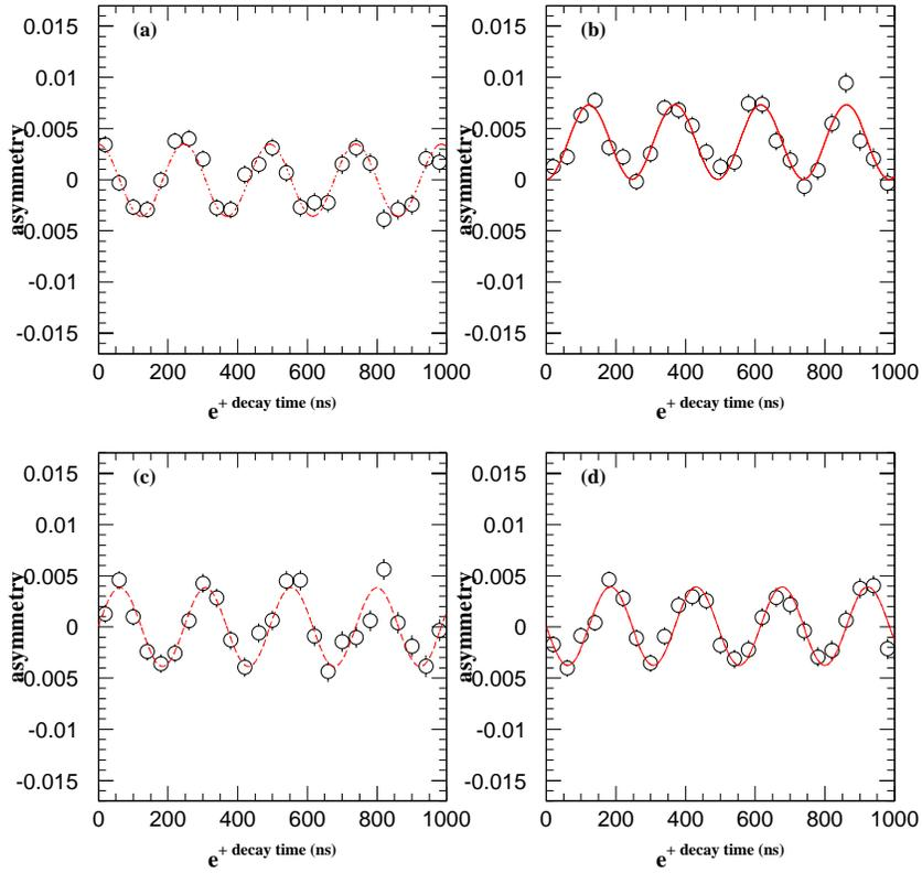
Figure 33: Example of MC studies on alignment calibration. Misalignments of (a)  $\epsilon_r = 1^\circ$ , (b)  $\epsilon_z = 1^\circ$ , (c)  $\delta_r = 1^\circ$  and (d)  $\delta_z = 1^\circ$  were artificially put in the simulation. The asymmetry of normalized positron time spectra are shown fitted with red expected curves.
