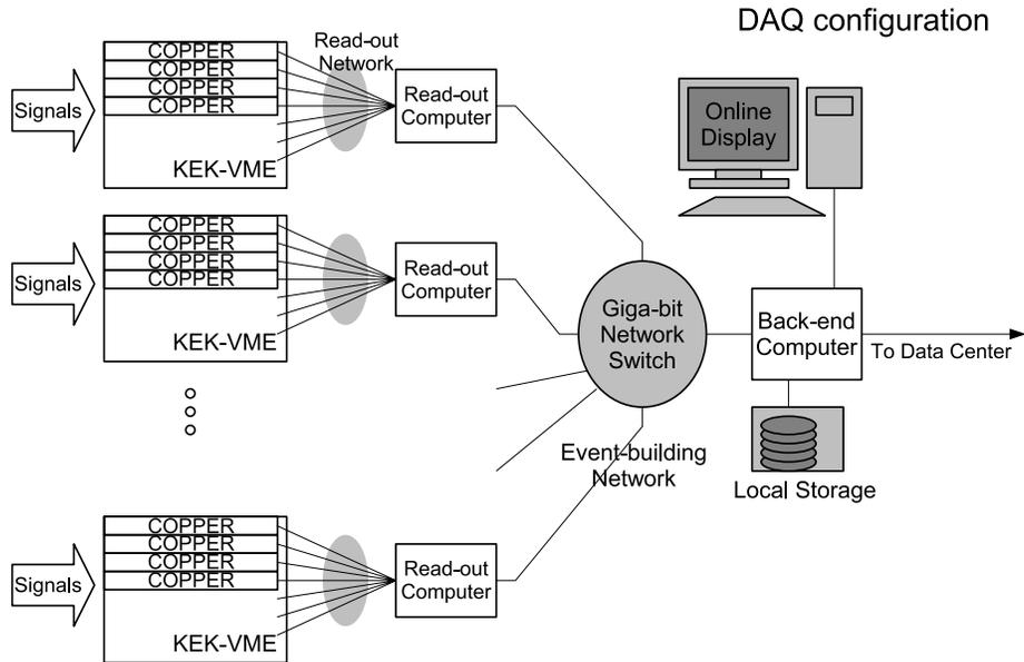
Figure 20: Data taking configuration with KEK-VME and COPPER scheme
