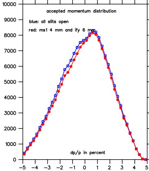
Figure 26: ZGOUBI result of the accepted momentum distribution for the 0.8 GeV/ $c$  beam.
