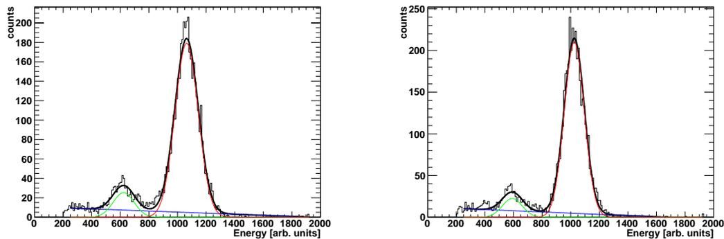
Figure 41:  $^{55}\text{Fe}$  spectrum recorded with a triple GEM prototype based on CERN foils for top (left) and bottom (right) strip readout. The full-energy photo peak and the argon escape peak are cleanly separated. The spectrum is fitted with two Gaussians and a linear background. The energy resolution of the photo peak is  $\sim 20\%$ , given by the FWHM of the peak.
