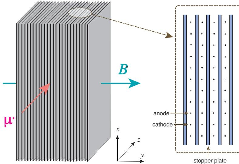
Figure 15: Muon stopper made of parallel plates which serve also as drift chamber cell structure.
