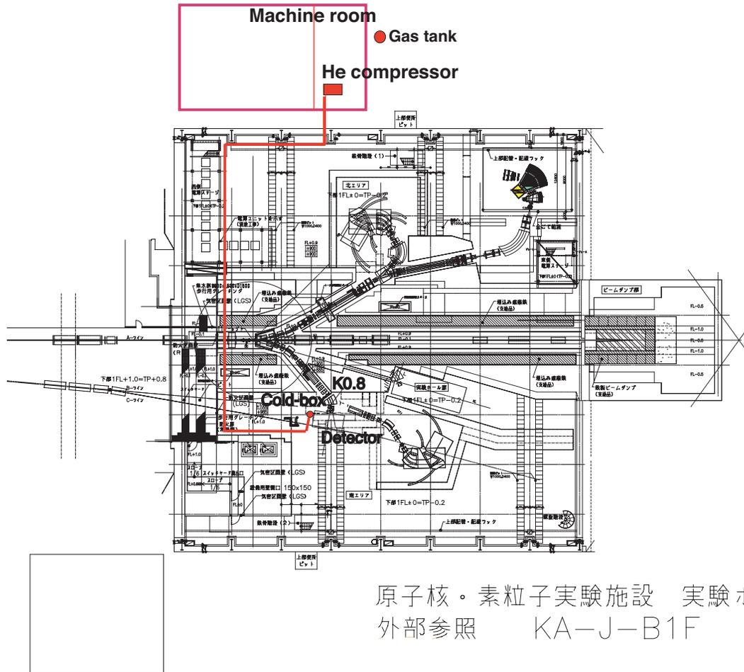
Figure 37: Layout of the superconducting toroidal spectrometer with its cryogenic system in the Hadron Experimental Facility
