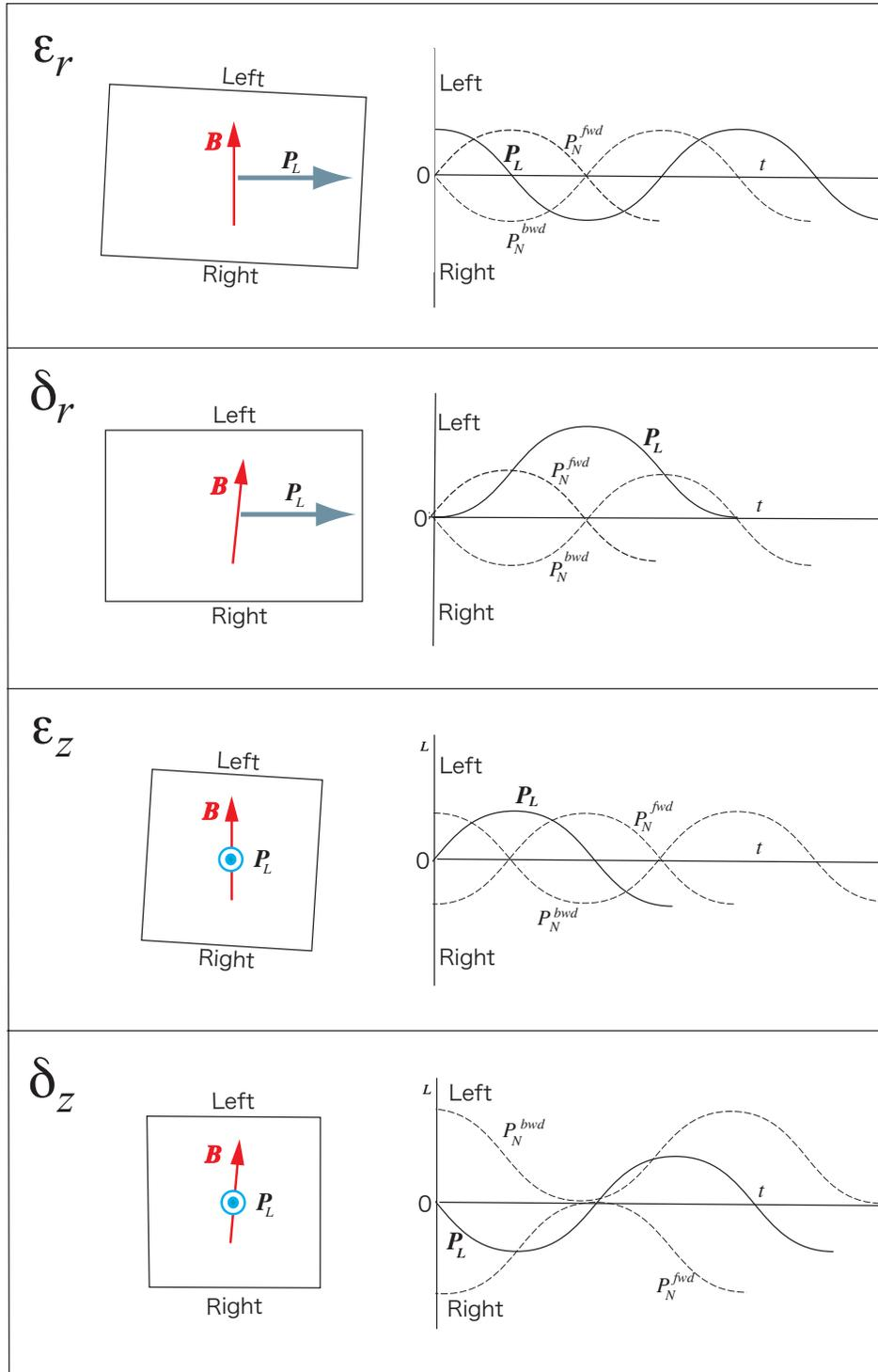
Figure 32: Calibration of polarimeter alignment and magnetic field direction. The longitudinal polarization  $P_L$  is utilized. Solid line show the asymmetry observed when the individual misalignment is present. Dotted lines are the spurious asymmetry in the main measurement due to  $P_N$  admixture. The time-integrated asymmetry is not  $fwd/bwd$  cancelling only for  $\delta_z$ .
