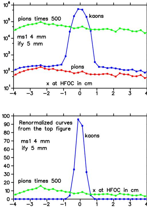
Figure 28: REVMOC result for the 0.8 GeV/c beam. Horizontal beam spots at HFOC for kaons and pions, logarithmic scale at the top and renormalized scale at the bottom. The pion distribution is wide due to scattering in the 30 cm long slits at IFY and MS1.
