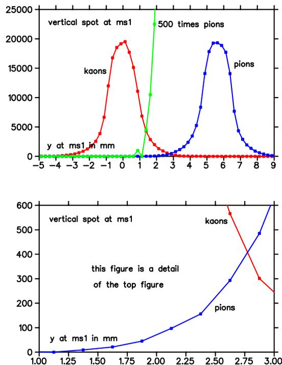
Figure 25: ZGOUBI result for the 0.8 GeV/c beam. The vertical beam spot at MS1 for kaons and pions. The green line shows the pion distribution multiplied by 500.
