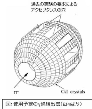
Figure 5: Schematic view of gamma detector
