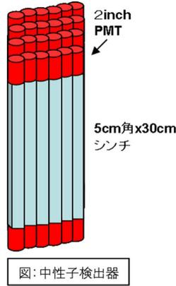
Figure 4: Schematic view of neutron counter
