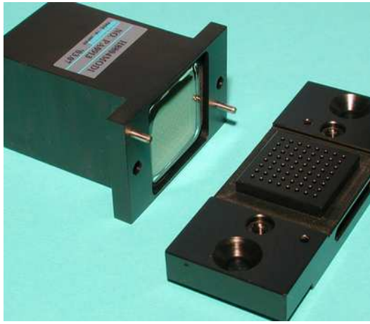
Figure 4: The 64 channel multianode PMT (H8804MOD-1) with alignment pins and a cookie.
