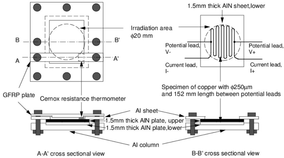
Fig. 3: Drawing of the sample and its retention developed in the beam line at FFAG accelerator facility in KURRI [13].
