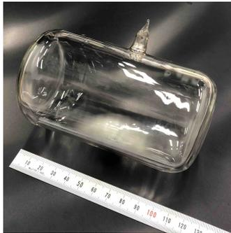
FIG. 22: A  $^3\text{He}$  spin filter with a dimension of  $\phi 6.5$  cm and 11.5 cm.
