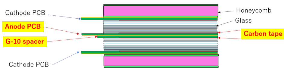
Figure 11: The MRPC structure.
