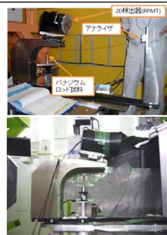
Two-dimensional TOF scintillation detector was installed at 600 mm away from the center of the analyzer unit, with keeping the reflection angle of the crystals. The reflected neutrons which wavelength of 6.61A were expected to reach the detector at 69.2ms. (see right photos)
