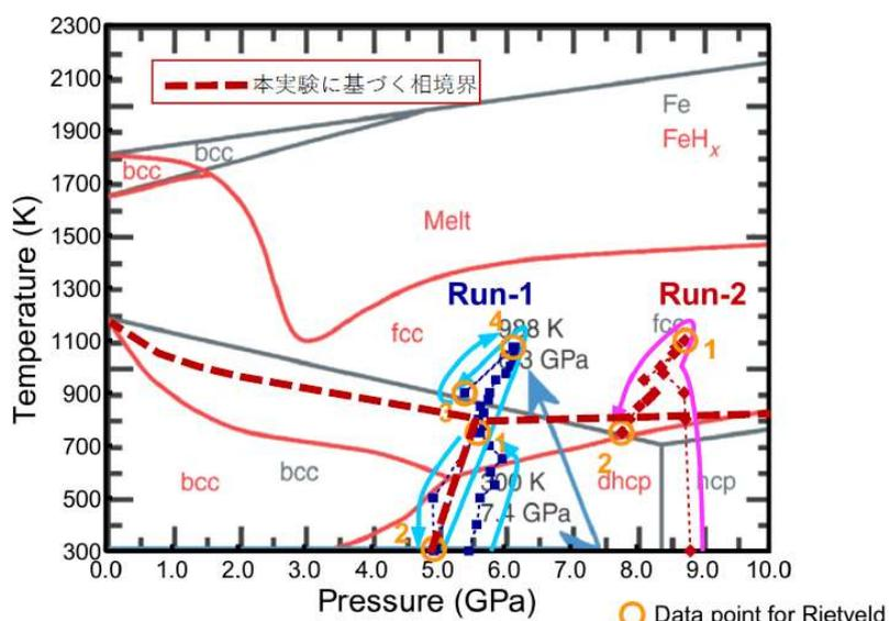
temperature for the first time. The phase transition and hydrogenation of iron were observed by dhcp-FeH<sub>x</sub> and fcc-FeH<sub>x</sub> phase, which are high pressure and high temperature phases of FeH<sub>x</sub>. We have conducted two separate runs. Run 1 was made in the pressure range around 6 GPa using the pressure cell for the cubic anvils with 10 mm truncated edge length. Run 2 was made at around 8 GPa using the anvils with 7 mm truncated edge length. The pressure-temperature paths
