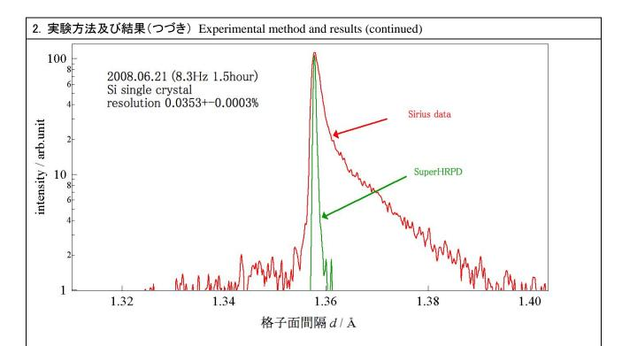
The measured Bragg reflection at d = 1.36 Å. In comparison, the same Bragg reflection obtained by the previous high resolution powder diffractometer *Sirius* (KEK – KENS) is shown.
