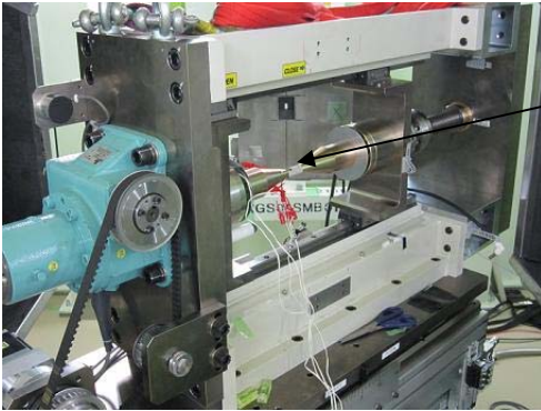
fig. 1. Photo of the experimental assembly, with the rock sample positioned at 45° to the incident beam.
