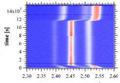
$\parallel$  scattering vector  $\parallel$  [1/Å] Figure: The central line represents the  $\beta$ -Zr 110 reflection, showing extinction and change of reflectivity upon plastic deformation at 8000 s.
