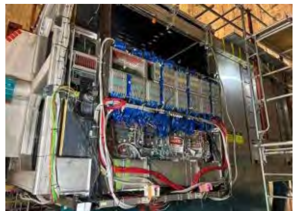
Fig. 7. A photo of the upgraded near detectors: SuperFGD, bottom HATPC, and 4 ToFs.
