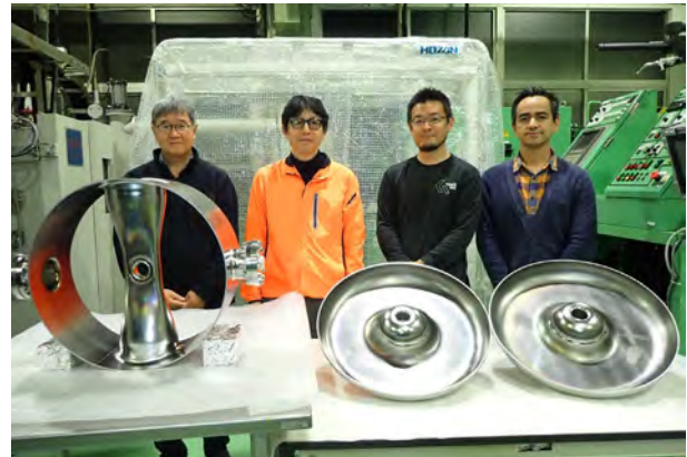
Fig. 6. Fabricated main parts of the prototype spoke cavity.
