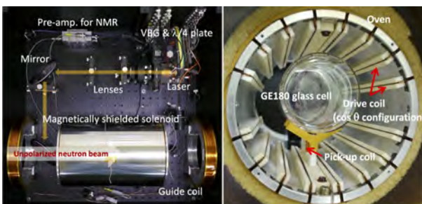
Fig. 2. Newly developed in situ SEOP polarizer system. Left: the SEOP system installed in the POLANO beamline. Right: NMR coils and a glass cell.
