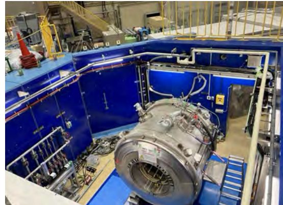
Fig. 4. The MRI magnet in H1 area of MUSE.
