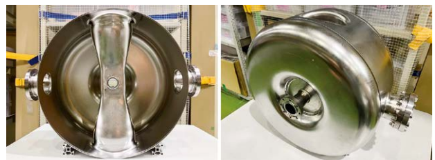
Fig. 8. [Left] After welding the body and one lid together. [Right] After welding the body and the other lid together.
