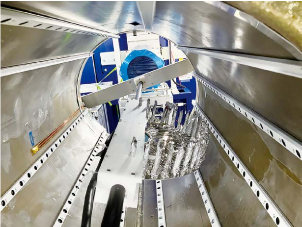
Fig.4. Setup for magnetic field measurement in the MRI magnet
