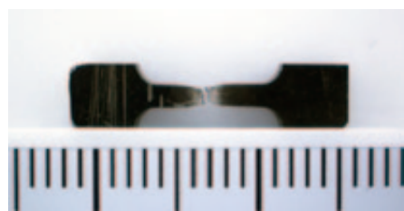
Fig. 2 The tensile specimen tested at RT (T91, 1.44 dpa).
