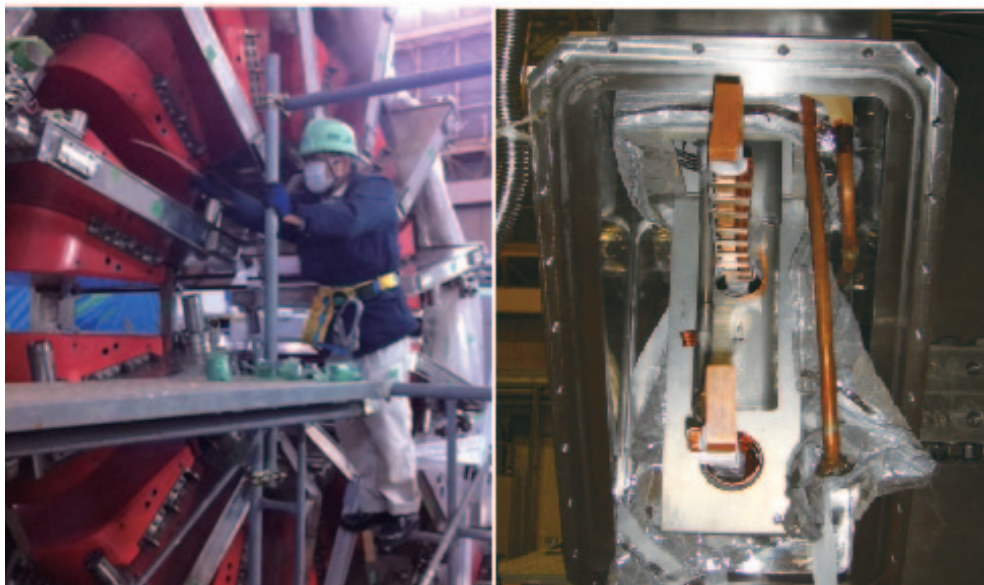
Fig. 3. Overview of the toroidal superconducting magnet (left) and the internal assembly (right).
