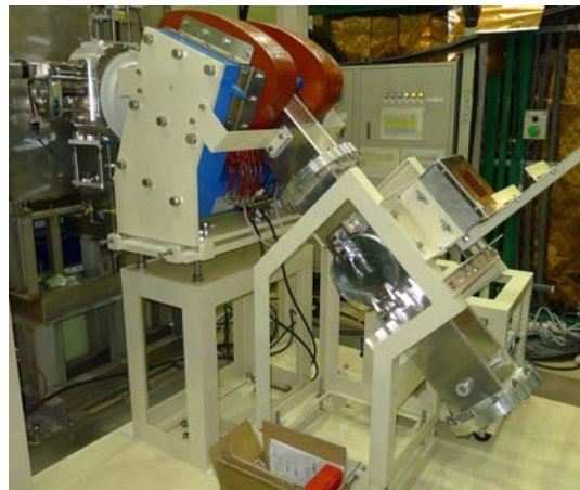
Fig. 1 Negative-muon-induced X-ray analysis system developed in this work.
