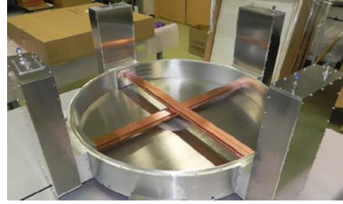
Fig. 1 Photograph of Straw tracker system prototype. 16 tubes for both X and Y coordinates were installed. The tube consists of 10 mm diameter and longer than 1 m length.
